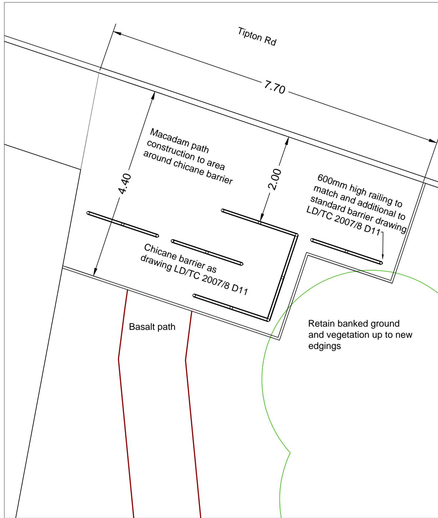
Detail plan A: Tipton Road entrance Anti motor cycle chicane barrier 1:50 @A1
